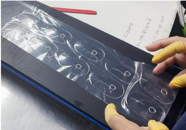
During the production of transparent products, the staff is requested to wear finger gloves to prevent the finger prints from affecting the next step
