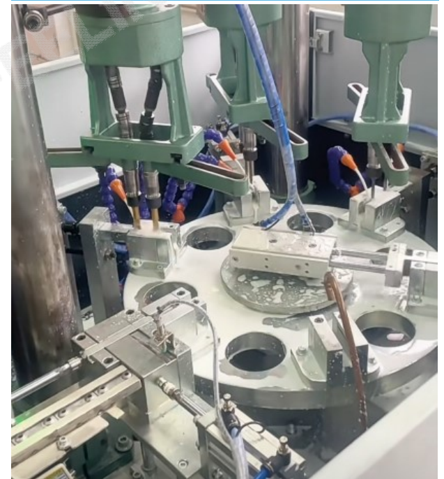
Fully automatic drilling and tapping integrated processing
