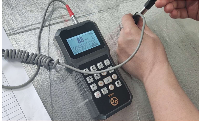
1: Raw material size and hardness testing
