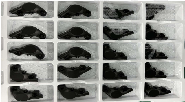
Assembly of semi-finished parts vacuum forming box transportation
